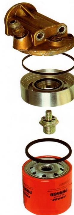
Ensure that the area around the oil filter housing is clean and remove the existing filter bowl. Place a tommy bar through the hole in the anchor screw boss (the part into which the long filter-retaining bolt screws) and remove the boss and splash plate.
